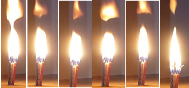
Fig. 1: Phenomenon of flickering and stratified flame.
